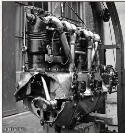
These photographs of a Benz Bz.III engine, taken to document severe damage to the front end, allow us to see many interesting details.
